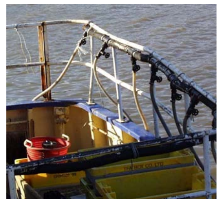
A simple wetting system coupled to the hosepipe
