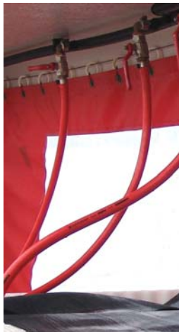
Below: Installed water taps make it possible to regulate the water flow and change the flow to different stacks.
