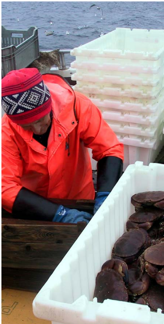
SE-40 boxes can store 38 - 40 kg of crabs. In small boats stacked boxes are very handy because of the saving of space when the boxes are stored.
