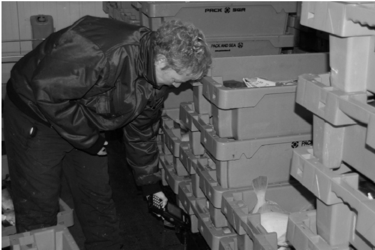
Figure 7 Using a hand held RFID reader to assign a fish box to a new owner. Low selectivity means that close range reading is necessary to select the right box (Case 2 fish auction). Photo: Ola Bø
